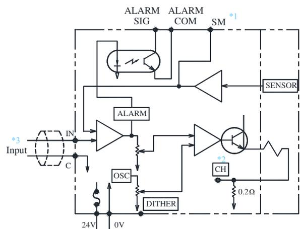
\*1 For "SM" terminal, external instruments should have input impedance of more than 10 kΩ.
